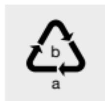
Observe the marking of the packaging materials for waste separation, which are marked with abbreviations (a) and numbers (b) with following meaning: 1–7: plastics/20–22: paper
