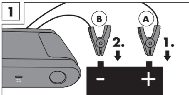
**⚠ WARNING!** As soon as the vehicle starts, remove the jump lead **10** from the portable jump starter with power bank **1** within 30 seconds and disconnect firstly the black battery clamp and then the red clamp from the battery poles. Otherwise, it could result in dangerous situations! Leave the vehicle engine running.
