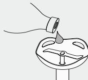
If you hear unusual noises during operation, e.g. squeaking or similar, apply a small amount of neutral cooking oil to the drive shaft of the hand blender ⑯.
