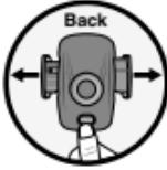
Press the **PRESS** button ⑦ on the rear of the device and the fixer grips ⑥ of the car cradle automatically move outwards.
