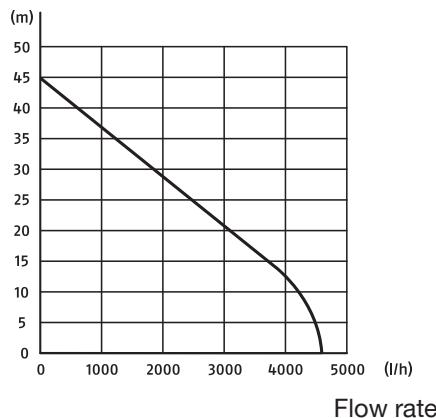
The maximum performance data is measured under optimal conditions (e.g. straight, direct outlet). Tighter hoses can reduce the output.
