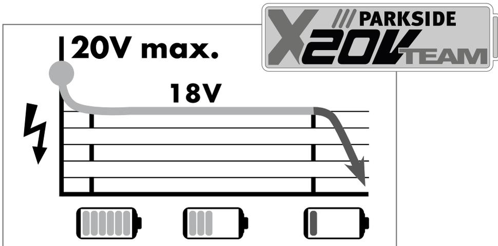
**All Parkside tools and the chargers PLG 20 A1/PLG 20 A2/PLG 20 A3 of the X20V Team series are compatible with the PAP 20 A1/PAP 20 A2/PAP 20 A3 battery pack.**
