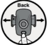
Press the **PRESS** button **7** on the rear of the device and the fixer grips **6** of the car cradle automatically move outwards.
