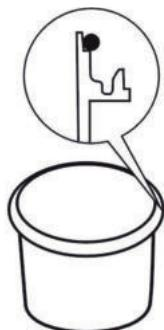
**! NOTE:** Position the large rubber seal on the upper edge of the filter barrel **[6]** (see Fig. left). Make sure that this does not move when you close the cover. If necessary you can also moisten the seal.
