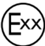
The e-Mark is a certification mark for the labelling of components requiring approval in motor vehicles and states that the necessary tests have been carried out and that an ECE component approval has been issued.
