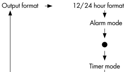
**Note:** If no button has been pressed for one minute, the LC display **[1]** returns to the output format.
