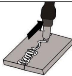
To forestall or reduce deformations that can happen during the material hardening process, it is good to fix the workpiece with a device. Avoid stiffening the welded structure to prevent cracks in the weld. These problems can be avoided if there is a possibility of turning the workpiece so that the weld can be carried out in two passes running in opposite directions.
