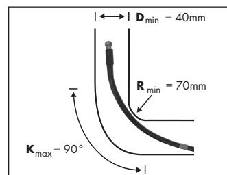
Designed for an operating/rated pressure of max. 150 bar.
