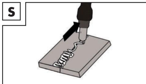
To forestall or reduce deformations that can happen during the material hardening process, it is good to fix the workpiece with a device. Avoid stiffening the welded structure to prevent cracks in the weld. These problems can be avoided if there is a possibility of turning the workpiece so that the weld can be carried out in two passes
