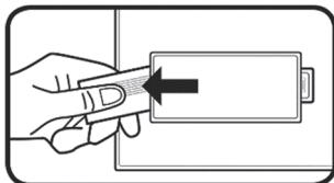
Remove the strip from the battery compartment (4) on the bottom of the bathroom scales. The bathroom scales are now ready to use.
