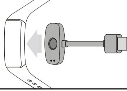
**(GB) (IE) (NI)** To start up the fitness wristband, keep the button pressed until the bar in the display has fully loaded, or connect the fitness wristband to the charging cable. If the bar does not appear after you have pressed the button for a long time, press the button briefly once.
