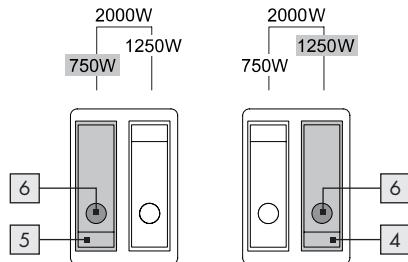
**Please note:** The indicator light [6] of the respective toggle switch [4] resp. [5] used will turn on during operation.
