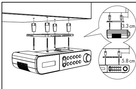
Using the supplied mounting plate **11**, you can install the product e.g. under a wall cupboard. Proceed as follows to mount the product:
