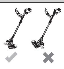
When adjusting the working positions, make sure that the protective cover 9 protects you from the cutting device.
