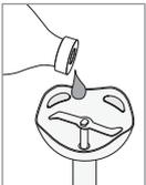
If you hear unusual noises during operation, e.g. squeaking or similar, apply a small amount of neutral cooking oil to the drive shaft of the blender **4**.
