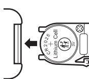
2. Replace the old battery with a new one. The positive pole (+) of the battery must be pointing upwards.
