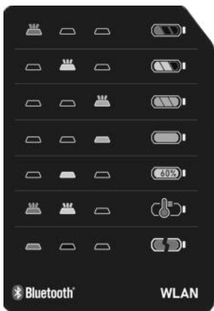
Control LEDs on the charger
