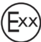
The e-Mark is a certification mark for the labelling of components requiring approval in motor vehicles and states that the necessary tests have been carried out and that an ECE component approval has been issued. The letters "xx" are placeholders and stand for the country where the licence was issued.
