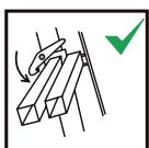
**GB** **IE** **NI** Locking devices shall be checked and be fully secured before use if not operated automatically.
