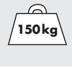
Maximum total load 150 kg. The weight of the user plus tools and other materials must not exceed 150 kg.
