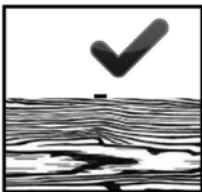
The crown of the staple or head of the nail should be flushed with the top of the material being fastened as shown.
