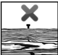
If the crown of the staple or head of the nail is not flush with the top of the material being fastened, it means it is too long. In this case, use the next shorter staple or nail for optimal results.
