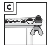
**GB** **IE** **NI** Place the correct sized pressure piece upside down beside the protruding end of the tube. Let the end of the tubing protrude from the tube to match the thickness of the large part of the pressure piece.
