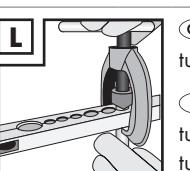
**GB** **IE** **NI** Make sure the cone point is centred on the tube and the flaring tool is locked on the tubing clamp.
