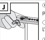
**GB** **IE** **NI** Loosen the screw and remove the pressure piece. The tube end should have a bubble look at this point.
