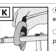
**GB** **IE** **NI** Position the flaring tool with the cone point entering the tubing end and centred.
