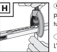
**GB** **IE** **NI** The cone point must be centred on the pressure piece. The flaring tool must be locked on the tubing clamp.
