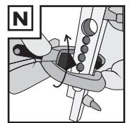
**GB** **IE** **NI** Remove the flaring tool. Inspect the tubing end. The flare should be even all around with no cracks or gaps. Remove the tubing from the clamp.
