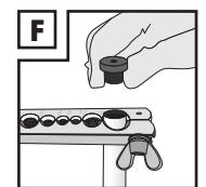
**GB** **IE** **NI** Turn the pressure piece over. Coat the pressure piece with a small amount of lubricant. Insert the pressure piece into the tube.
