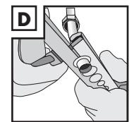
**GB** **IE** **NI** Tighten the wing nuts tightly. Keep the halves of the tool parallel to each other as you tighten. Tighten the wing nuts with a suitable tool.
