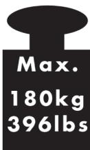
This symbol indicates that the bathroom scales cannot bear weights over 180kg / 396lb. Otherwise, the bathroom scales could be damaged and there is a risk of injury.
