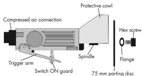
Compressed air supply and connection. Use filtered, lubricated, and regulated compressed air only. The following figure illustrates the correct way
