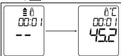
on the display and the end of measurement is indicated with a short beep (when the key tone is activated). When the measurement type symbol stops flashing, the next measurement can be taken. This takes approx. 5 seconds.
