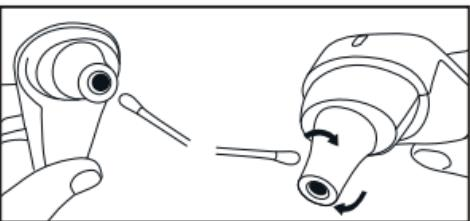
Use a soft cloth or a cotton bud which can be dampened with antiseptic, alcohol or warm water to do so.
