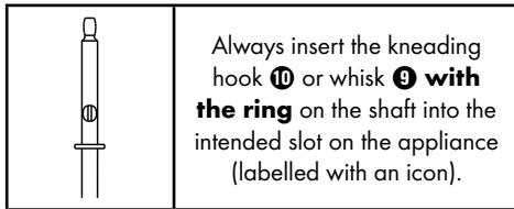
Always insert the kneading hook ⑩ or whisk ⑨ **with the ring** on the shaft into the intended slot on the appliance (labelled with an icon).
