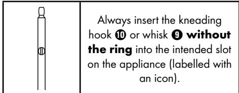
Always insert the kneading hook ⑩ or whisk ⑨ **without the ring** into the intended slot on the appliance (labelled with an icon).
